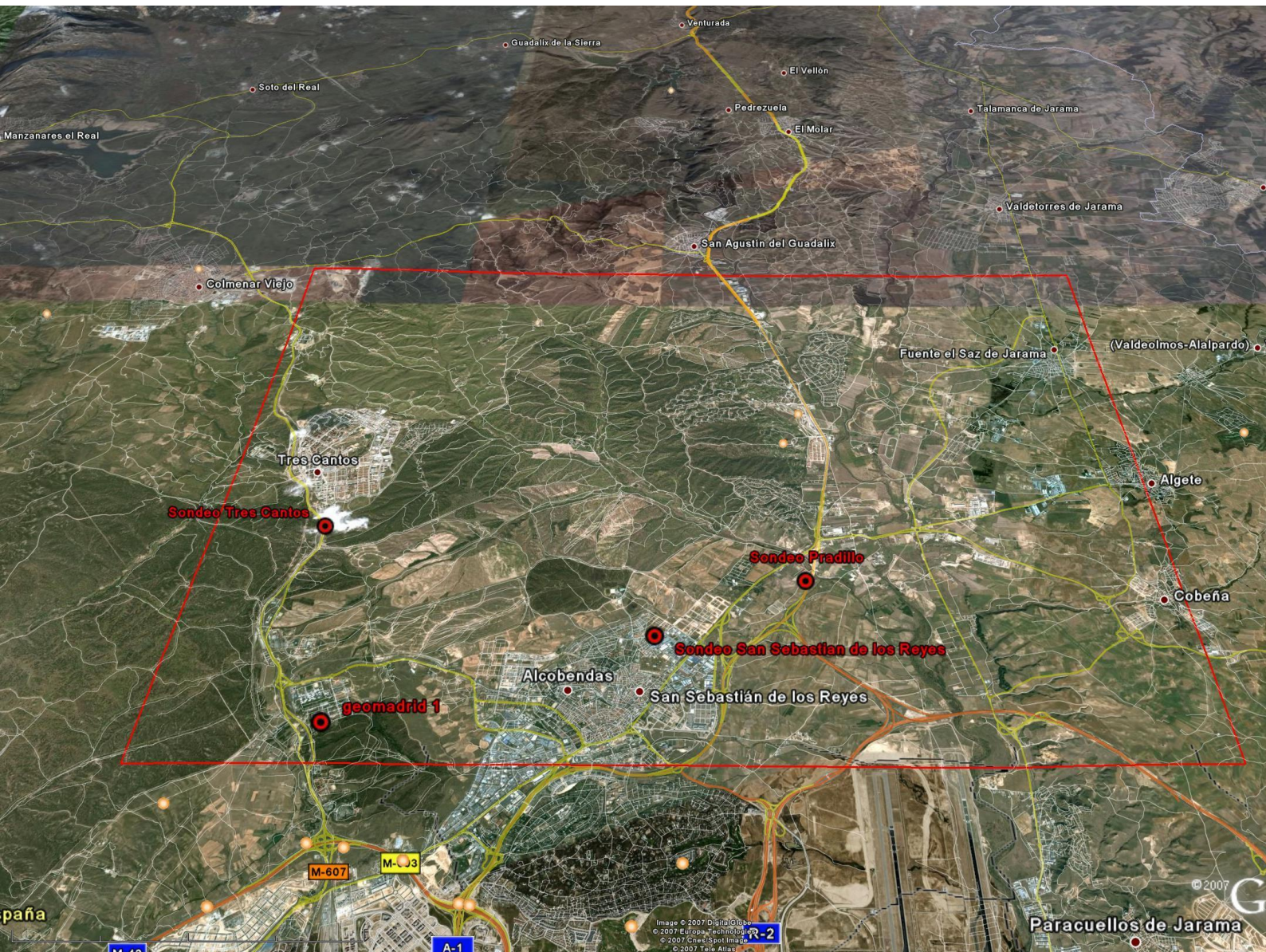
Figure 1 - Madrid Geothermal License Area – located 25 kms north of the City and covering over 300 square kms. The 8 MW Geo-Madrid Project is in the left foreground. Other potential projects for application of district heating on the Madrid tenement area are San Sebastian de los Reyes (middle foreground) and Tres Cantos (left middle-ground).
