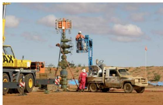
Figure 3 - Paralana 2 preparation for injectivity test
